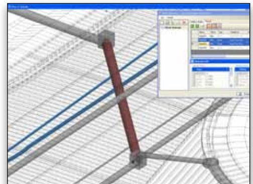
*Clash detection of utilities and drainage using ProjectWise Navigator.*
